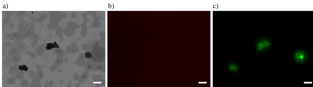
Figure 6-18. Fluorescence images of bi-functional microparticles functionalized only with Oregon green , a) in bright field, b) excited using green filter and c) fluorescence from Oregon green , at pH 7. Scale bar – 5 \mu\text{m} .
