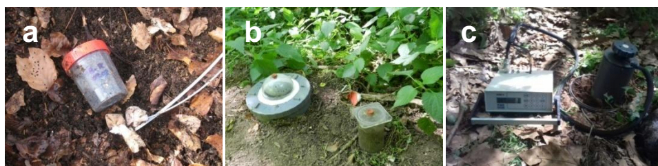
Figure 2.3 (a) Soil incubations to measure soil N processes, (b) soil chambers to measure natural N 2 O emissions and denitrification, and (c) EGM-4 chamber associated to an IRGA. Source: Anna Lupon, Sílvia Poblador, and Francesc Sabater.
