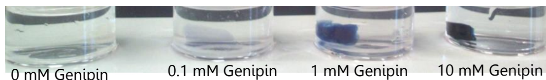
Figure 4.19. 8wt % Gelatin gels, crosslinked with different amounts of Genipin, inside a citrate/phosphate buffer solution of pH 7.
