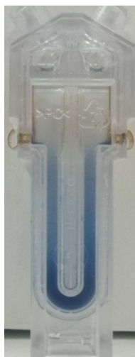
Figure 4.62. Microgels, here blue as crosslinked with genipin, started to sediment after few seconds inside the measuring cell, making zeta potential measurement not possible.
