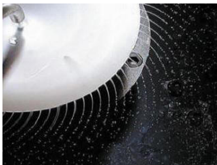
Figure 1.19. Spinning disk showing jets and drop break up. (Figure reproduced from (Southwest Research Institute Website, 2015)).
