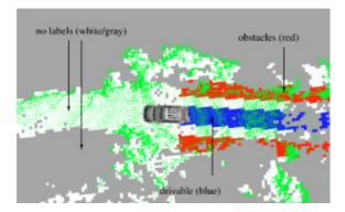
**Figure 8.1.:** Thrun et al. (2006): Data labelling through human driving. Traversed areas (blue) are assumed as *drivable* and two stripes with a defined distance to the left and to the right are assumed as *non-drivable* (red).
