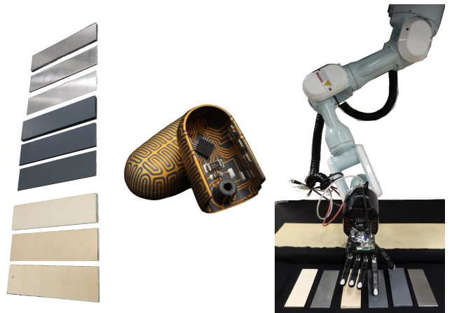
Fig. 4. Left: the material used in experiments. Middle: the fingertip MID tactile sensor. Right: a Mitsubishi PA-10 robot arm and the Shadow dexterous hand equipped with tactile sensors.
