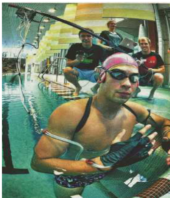
Fig. 3 a) Setup to measure static pressure on two sides per hand of a swimmer; 3 b) setup details
