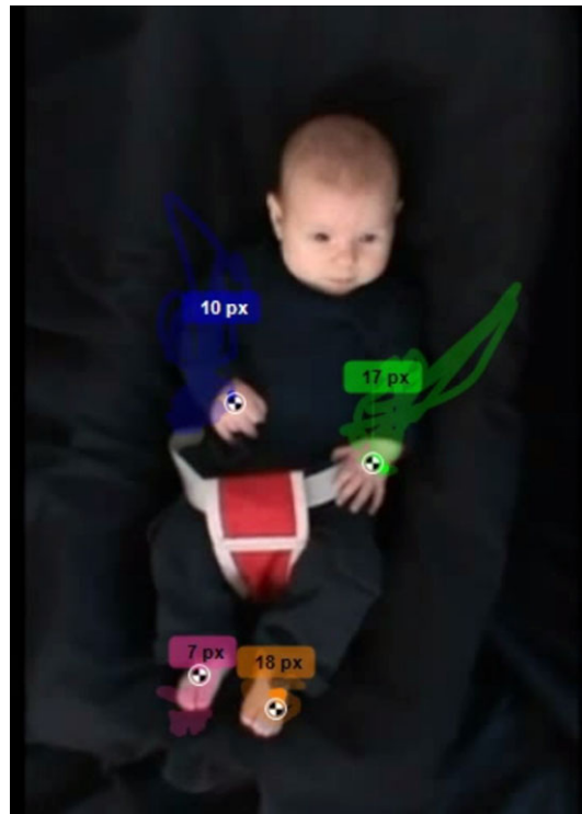
Figure 2. Screenshot of Kinovea in use for coding an infants' limb activity. The coloured rectangles above each limb indicate the number of pixels traveled by the limb.
