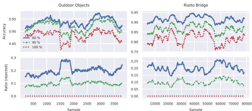
Fig. 3. Accuracy and reject ratio over time according to different reject thresholds for SAM, shown for the datasets Outdoor Objects and Rialto Bridge . Thresholds are chosen such that 100 %, 90 % and 80 % of points are accepted. Accuracy and ratio are calculated over a sliding window that contains 10 % of the respective dataset’s total number of samples. Note the abrupt, temporary drop in accuracy for Outdoor Objects and the corresponding increase in the number of rejected points for samples 1700 to 2200.
