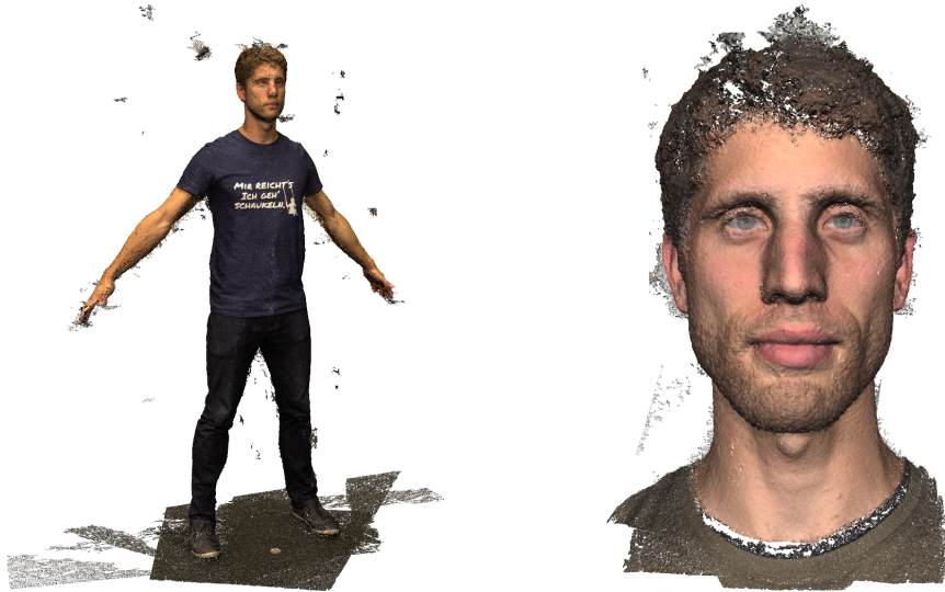
Figure 4.2: Examples of the computed point clouds from our 40 camera full-body scanner (left) and 8 camera face scanner (right).
