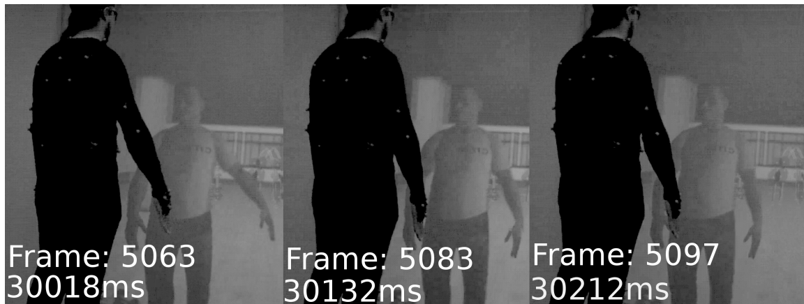
Figure 2.8: Example frames from one of the latency test videos (highest quality character with shadows). The left image shows the user’s arm approaching the lowest point. The image in the middle shows the turning point of the real arm, the picture on the right shows the turning point of the virtual arm, while the real arm already moves upwards.
