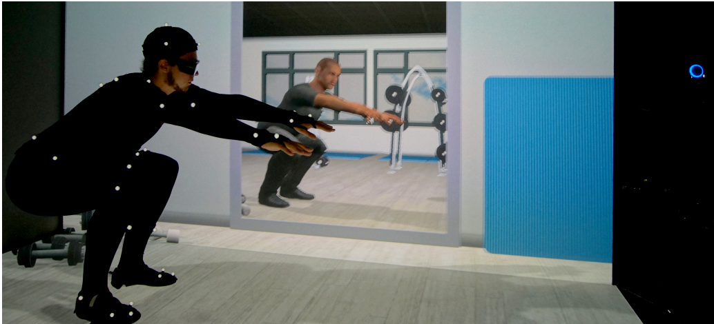
Figure 2.4: Real-time feedback using a virtual mirror requires an immersive Virtual Reality environment that provides full-body motion capturing, motion analysis, and realistic character rendering at a low end-to-end latency.
