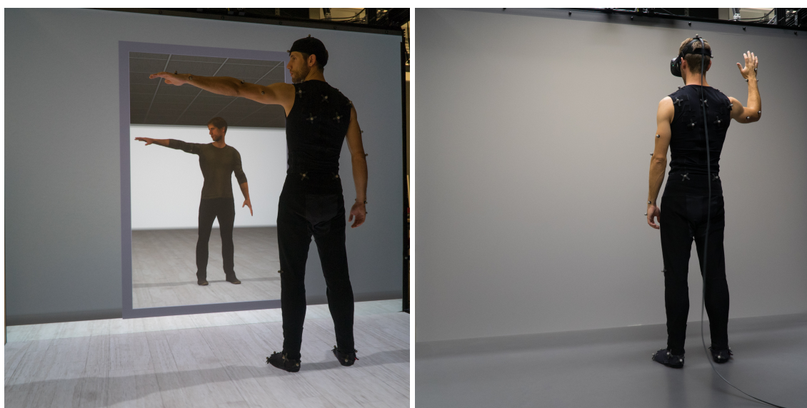
Figure 5.1: The two VR setups used in the study. The participants were immersed in the same virtual room with a virtual mirror using an L-shape part of a CAVE (condition CM1, left) and a HMD (condition CM2, right). The participants wore a motion capture suit to track their full-body motion by a passive marker-based motion capturing system. Note that in the L-shape condition the participants had to wear 3D glasses for stereoscopic visualization (not shown in the image).
