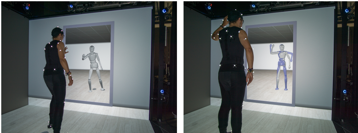
Figure 3.1: Left: The basic virtual mirror scenario consists of an empty room and a simplistic mirror avatar. Right: The extended scenario employed in the experiment, where the target movement is shown by a semi-transparent blue “ghost character”.
