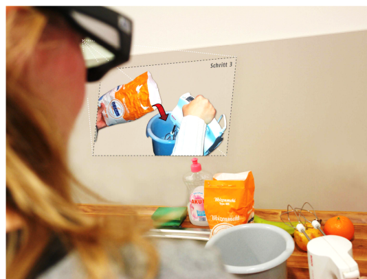
Figure 1: ADAMAAS will provide situation-, user-, and action-specific feedback on a transparent virtual plane superimposed on the user's field of view.
