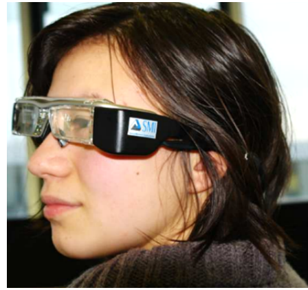
Figure 2: The ADAMAAS AR-Eyetracking System designed by SensoMotoric Instruments (SMI)
