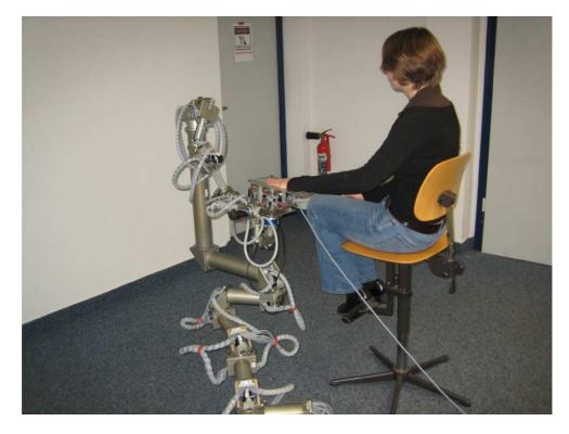
Figure 4.7: Shear-Force Display mounted on ViSHaRD 10.
