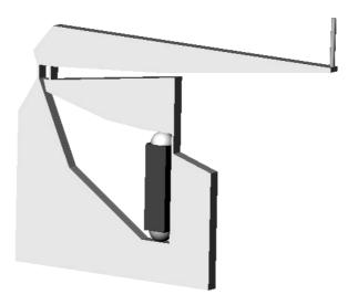
Figure 2.10: Final combined lever system with stack piezo
