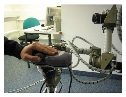
Figure 4.8: VirTouch Mouse mounted on ViSHaRD 10.
