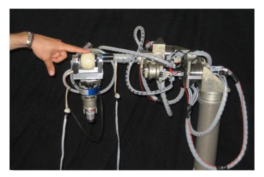
Figure 4.6: Slip-Friction Display mounted on ViSHaRD 10.
