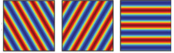
Fig. 5. Stripe-cell receptive fields can be modeled as rotated sine-functions in the two-dimensional plane [21].
