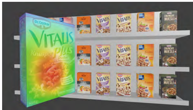
Figure 1: The presented approach creates realistic heat maps for objects that have been moved around and inspected from all sides in real-time with a high-quality. Here the example of a product picked from a shelf of a virtual supermarket (see also Figure 5).
