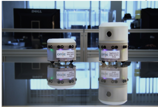
Fig. 5. Autonomous Mini Robot (AMiRo) in two different version. Left: Basic Robot. Right: Mounted Kamera Tower
