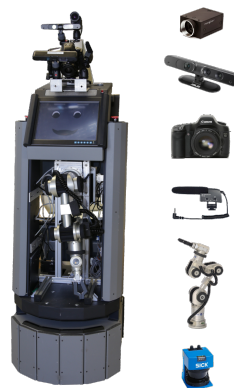
Fig. 1. ToBI with its components: camera, 3D sensors, microphone, KATANA arm and laser scanner.
