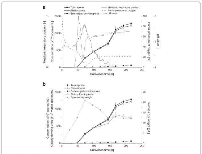
Figure 3 Cultivation of *B. bassiana* in a 2 L stirred tank reactor. The figure shows the mean (±SD) concentrations of TS, BS and SCS. (a) Process parameters. (b) Correlation of spore counts with biomass and mean (±SD) CFU. In each case, standard deviations resulted from two technical replicates.
