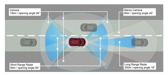
**Figure 1.1:** Sensor Fusion of a Driver-Assistance System: The blue-filled cones illustrate the working range of short-range and long-range radar systems. Cones with blue dotted outlines indicate the working range of four cameras to build a 360-degree view. The orange-colored outlines depict the working range of a stereo camera system. The small white-colored cones signify the working range of 12 ultrasonic sensors.
