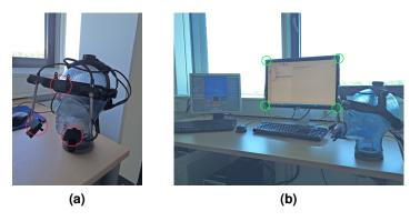
**Figure 9.6:** Experimental Setup: (a) depicts the EyeLink II with its three cameras. The cameras are marked with red circles. (b) portrays the experimental setup. The LEDs at each corner of the screen are marked with green circles.
