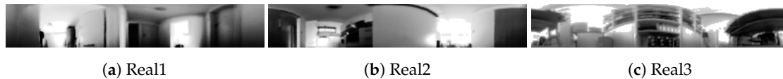
Figure 19. Low-resolution, unfolded panoramic images acquired by our robot. These images are created by reprojecting, blurring and histogram-equalizing the images in Figure 18. In this work, we use such images to calculate the image distances described in Section 2.2.4. Our robot also performs visual navigation with images of this type.
