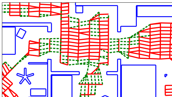
Figure 12. The effect of edge classification on the map graph from Figure 5. Edges classified as crossing a room border are drawn as green, dashed lines. While most room-border edges are classified correctly, we also note some false-positive results within the rooms.
