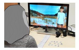
Figure 2: Overview of the setup (as seen from the rear camera). Touchscreen PC with eye tracker mounted below. High-fps face camera recording from below the screen. The physical item list and the items to allocate on it in preparation for the game are visible on the desk. The microphone is occluded by the participant (anonymized). Start of interaction.
