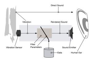
Figure 2: Auditory Augmentation model: Structure-borne sounds are sensed with a contact microphone, filtered according to parameters defined by an external data source an then played back. The filtered signal shapes the resulting interaction sound as it blends with the original sound.
