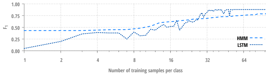
Fig. 4. Early learning behavior, averaged over 10 random folds. HMMs outperform the LSTM network where very little training data is available, while the latter performs better with more than 28 training sequences. Note that the x-axis is scaled logarithmically.
