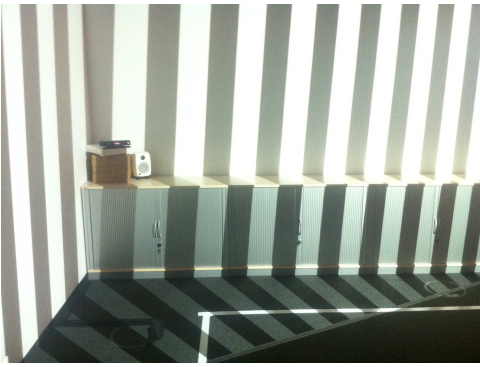
Fig. 3: Projected gray code to gather correspondences to the depth camera's 3D points.
