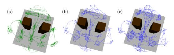
Fig. 7.5: (a) Training data recorded for evaluation of the local bootstrapping heuristic. (b,c) Generated navigation graphs G by ITM algorithm without and with local boostrapping ( $\delta = 4$ ).
