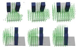
Fig. 3.11: The reachable workspace (green dots) after kinesthetic teaching of obstacle setup II. From left to right, the tutor provided training data only in 1, in 4 or in 21 areas of the workspace, respectively.
