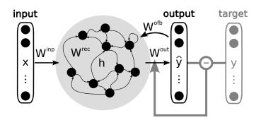
Fig. 3.3: The reservoir network architecture with respective input  $\mathbf{x}$ , hidden  $\mathbf{h}$ , and output  $\mathbf{y}$  layer. Learning affects only the output weights  $W^{\text{out}}$ .
