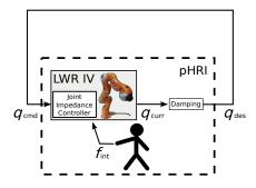
Fig. 4.1: Implementation of the required gravity compensation controller  $\pi_q$  according to Sect. 2.3.1. It utilizes the lowlevel joint impedance controller of the LWR IV and an additional damping term.
