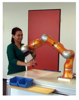
Fig. 1.1: Close physical interaction between human and the force-controlled KUKA Lightweight Robot IV.
