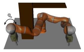
Fig. 4.17: Example for a consistent combination of redundancy resolutions  $(L_3-R_4)$  in left and right training area but with data very close to the LWR IV's joint limits.
