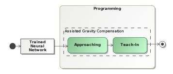
Fig. 2.8: Proposed interaction workflow for assisted *PROGRAMMING* using the trained neural network embedded into the hierarchical controller. Transition between the individual sub-stages *APPROACHING* and *TEACH-IN* is again realized based on the triggers on\_affected and on\_converged.
