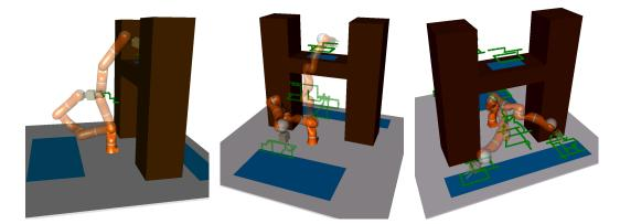
Fig. 8.3: Illustration of the redundancy resolutions for some of the K = 8 training areas recorded during the *CONFIGURATION* stage for the simulated 9-DoF manipulator. The recorded task space positions  $\mathbf{x}_l^{(k)}$  are plotted as green dots and the selected initial joint configurations  $\mathbf{q}_{\text{fixed}}^{(k)}$  are visualized with a transparent robot, respectively.
