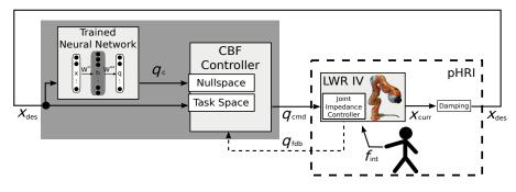
Fig. 5.2: Implementation of the proposed assisted gravity compensation controller concept from Sect. 2.3.3. The task space interaction controller  $\pi_x$  is implemented based on the low-level joint impedance controller of the KUKA Lightweight Robot IV and an additional damping term.
