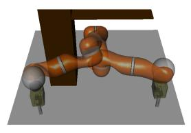
Fig. 4.13: Example for inappropriate combination of redundancy resolutions in left and right training areas.
