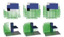
Fig. 3.10: The reachable workspace (green dots) after kinesthetic teaching of obstacle setup I. From left to right, the tutor provided training data only in 1, in 4 or in 12 areas of the workspace, respectively.
