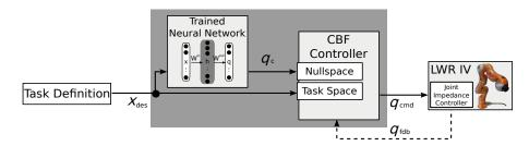
Fig. 3.1: Implementation of the *hierarchical control* concept with the learned neural network embedded into the control architecture.
