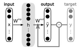
Fig. 3.4: The ELM learning scheme consisting of a single hidden layered feed-forward neural network with. Again learning affects only the output weights W<sup>out</sup>.
