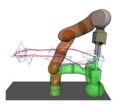
(b) Constructed navigation graph G and exemplary planned path from position (1) to same Cartesian position but with different end-effector orientation.
