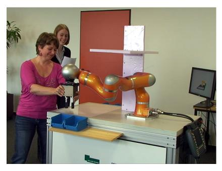
Fig. 4.8: Participant of the FlexIRob@Harting study during the *CONFIGURA-TION* phase teaching the LWR IV redundancy redundancy resolutions in the second training area of the confined workspace.
