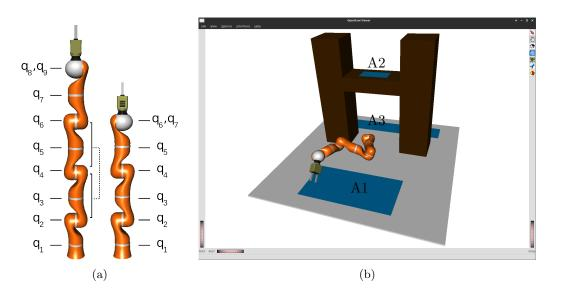
Fig. 8.2: Experimental setup used in this chapter: (a) Illustration of the simulated 9-DoF manipulator in comparison to the simulation model of the original KUKA Lightweight Robot IV. The duplicated links and joints are indicated. (b) Simulation environment and confined workspace consisting of different obstacles and three relevant working areas A1, A2 and A3 with the robot being mounted at the center of the plane.
