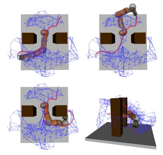
Fig. 7.7: The navigation graph G generated from the interaction data during the CONFIGURATION stage as shown in Fig. 7.5, and exemplary planned paths executed by means of the *hierarchical control* architecture embedding the learned redundancy mapping  $\mathbf{q}_c(\cdot)$ .
