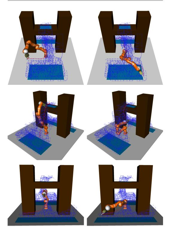
Fig. 8.4: Resulting navigation graph and exemplary planned paths after teaching the simulated 9-DoF arm.
