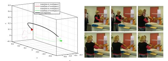
(a) Test person recording training data with only a low variance and guiding the robot arm through a kinematic singularity. As a result, the accuracy of the performed test trajectory (should be a straight line in-between the two areas of the workspace) is poor.
