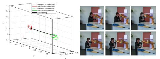
(c) Test person providing good training data with an appropriate variance and a valid combination of postures in both areas of the workspace. As a result, the robot is able to perform the test trajectory between the training areas with a high degree of accuracy.
