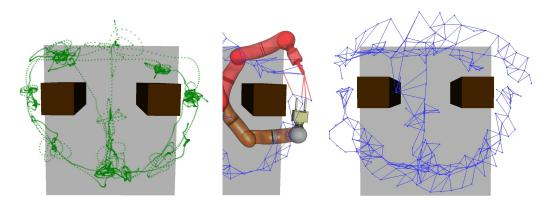
Fig. 7.3: Left: Recorded data from a training session during which the robot has been moved twice or more to same areas but with different redundancy resolutions. Center: Marked edge candidates between such areas that the standard ITM algorithm would connect but that can be detected as invalid using the joint space criterion. Right: The ITM learned from the training data with the joint space criterion included in the learning.
