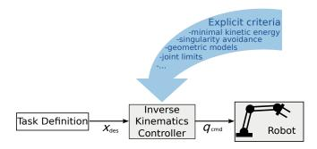
Fig. 2.1: Sketch of traditional approaches to redundancy resolution such as task augmentation and null-space projection methods. Besides an explicit definition of a task, explicit analytical criteria are required to resolve the manipulator's redundancy.
