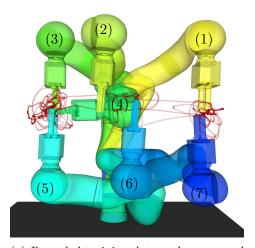
(a) Recorded training data and corresponding robot configuration in seven reelveant areas of the combined translational-rotational task space.
