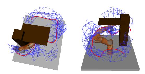
Fig. 7.8: Another illustrative result of the generated graph G and exemplary planned paths in a different obstacle setup.
