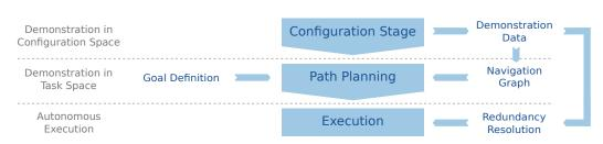
Fig. 7.1: Schematic view on the changed high-level interaction course (cf. Fig. 2.3 for comparison). The demonstration data gathered during the *CONFIGURATION* stage is exploited for both inference of a redundancy mapping and constructing a navigation graph in task space. After definition of a goal in task space, the latter is utilized for planning a safe task space trajectory, and the latter to execute this according to the demonstrated environmental constraints.
