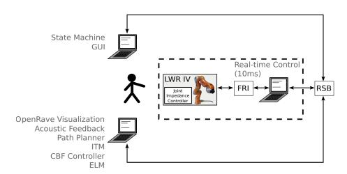
Fig. A.1: Illustration of the FlexIRob system including the KUKA Lightweight Robot IV, two PCs and a tablet PC for a graphical user interface.
