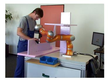
Fig. 5.1: A shop-floor worker from Harting [24] interacting with the FlexIRob system during the *PROGRAMMING* stage. He teaches a 3-D trajectory in a confined workspace while already being assisted by the robot's control system to avoid the static obstacles in the scene [22].
