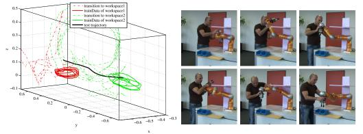
(b) Test person recording training data with a high variance but having problems guiding the robot arm from one area of the workspace to the other. Nevertheless, the performed test trajectory is more or less a straight line in between the two areas of the workspace.
