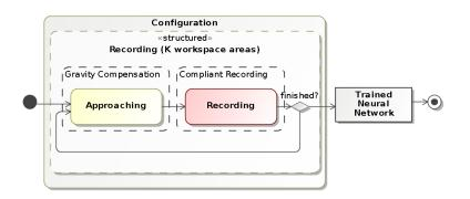
Fig. 2.5: Proposed interaction workflow for kinesthetic teaching of redundancy resolutions during *CONFIGURATION*. Transitions between the individual substages are realized based on the triggers on\_affected and on\_converged.
