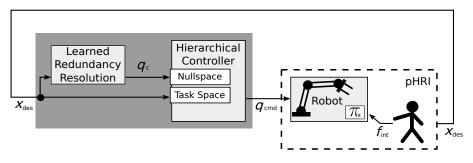
Fig. 2.7: Proposed assisted gravity compensation controller for the *PROGRAM-MING* stage following the demonstration-in-task-space strategy as discussed in Sect. 2.2.2. Utilizing the low-level controller  $\pi_x$  it allows free interaction with the robot's end-effector while controlling the redundancy resolution according to the learned function  $\mathbf{q}_c(\cdot)$ .
