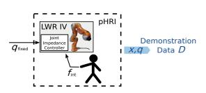
Fig. 4.2: Illustration of the proposed *compliant recording* controller  $\pi_{\rm rec}$ . It refers to the LWR IV's joint impedance controller and allows physical deflection only locally for recording consistent training data as proposed in Sect. 2.3.1.
