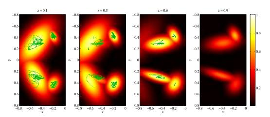
Fig. 6.5: Illustration of the learned confidence model C from the training data shown in Fig. 6.3. C is visualized in different heights z = (0.1, 0.3, 0.6, 0.9) of the robot's workspace for the parameter d = 15.
