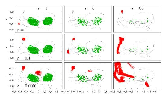
Fig. 3.13: Illustration of the encountered collisions during evaluation of the ELM networks in setup I, depending on regularization parameter  $\varepsilon$  and sub-sampling *s* of the training data. It plots the training data (green), the target trajectory (black dotted), and the robot positions  $\mathbf{x}_{curr}$  which caused collisions (red).
