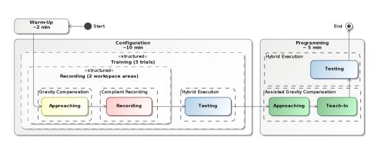
Fig. B.1: Illustration of the interaction workflow during the FlexIRob@Harting study, exemplarily for the assisted group (group A). After a short warm-up phase, the *CONFIGURATION* stage is repeated three times for each participant, each followed by a testing stage. The teach-in of the *PROGRAMMING* phase is done once and then replayed as feedback about teaching success to the user.
