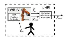
Fig. 5.3: Alternate implementation of  $\pi_x$  employing an external admittance controller.
