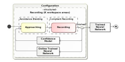
Fig. 6.1: Illustration of the proposed adoptions to the interaction workflow for kinesthetic teaching of redundancy resolutions during the *CONFIGURATION* stage. During *APPROACHING* the proposed *assistance blending* controller is utilized, embedding the online trained neural network and a confidence model in the control architecture.
