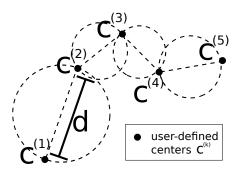
Fig. 3.5: Two-dimensional illustration of how the distance parameter d is obtained. The Thales circles of  $(\mathbf{c}^{(1)}, \mathbf{c}^{(2)}), (\mathbf{c}^{(2)}, \mathbf{c}^{(3)}), (\mathbf{c}^{(3)}, \mathbf{c}^{(4)})$  and  $(\mathbf{c}^{(4)}, \mathbf{c}^{(5)})$  are the only ones fulfilling the right-hand side of Eq. (3.18). The value of d is given as the diameter of the largest among those.
