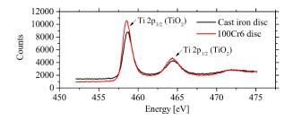
Figure 7: Material analysis with X-ray photoelectron spectroscopy inside the running marks of a 100Cr6 and a cast iron disc after a disc-disc test run with food-tech-oil, 1wt% T805 particles, 0.5 wt% Estisol<sup>®</sup> 242, 0.15 wt% oleylamine and 0.15 wt% Pluronic<sup>®</sup> RPE 2520. Titanium dioxide could be detected on both disc surfaces even after cleaning them with a 1:1 mixture of petroleum ether and acetone in an ultrasonic bath for two minutes. The same discs were imaged in Figure 8.
