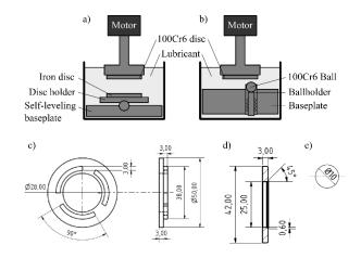
Figure 1: In the present study, we used 100Cr6-disc vs. cast iron disc contacts to evaluate friction coefficients (a) and 100Cr6 ball vs. disc contacts measure the anti-wear performance of our lubricants. c) Drawing of the segmented cast iron disc (total active area: 247 mm<sup>2</sup>) d) Drawing of the LS2542 100Cr6 axial bearing disc. e) Drawing of the 100Cr6 ball. All discs were lapped before use to generate planar surfaces.
