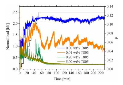
Figure 11: Friction coefficients in dependence of different concentrations of T 805 nanoparticles with 15 wt% oleylamine and 15 wt% Pluronic<sup>®</sup> RPE 2520 with reference to the particle concentration. The Estisol 242 concentration is equal to the particle concentration with the exception of the 5 wt% T 805 run, where 2.5 wt% Estisol<sup>®</sup>242 were added.
