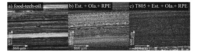
Figure 14: Micrographs of the 100Cr6-discs after disc-ball experiments. For better readability, the abbreviations Est. = 1 wt% Estisol<sup>®</sup>242, Ola. = 0.15 wt% oleylamine, RPE = 0.15 wt% Pluronic<sup>®</sup> RPE 2520 were used.
