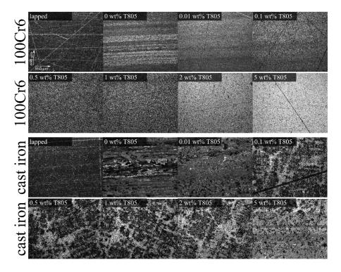
Figure 12: Micrographs of the discs involved in experiments to find the optimal concentration of  $TiO_2$  particles in the base oil. The least amount of wear was found for 0.5 wt% T 805 and 1wt% T 805 on the 100Cr6 discs and for 0.1 wt% to 1 wt% T 805 for the cast iron discs.
