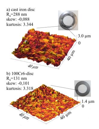
Figure 2: Photographs of the two discs that make up the tribocontact in this work and their surface parameters after lapping, obtained via 40x40µm<sup>2</sup> atomic force microscopy scans.
