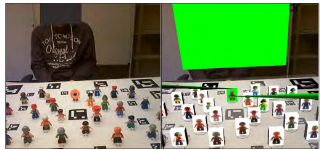
Figure 6: Study scenario from the view of one interaction partner. The participant wearing the eye tracker is currently fixating on a figure. On the left, the fixation is depicted in a still from a gaze video generated by the SMI software: the interpretation of the fixated figure is up to the human viewer. On the right, the 3D situation model is aligned to the perspective of the eye tracker and the target figure is determined and highlighted by our software.
