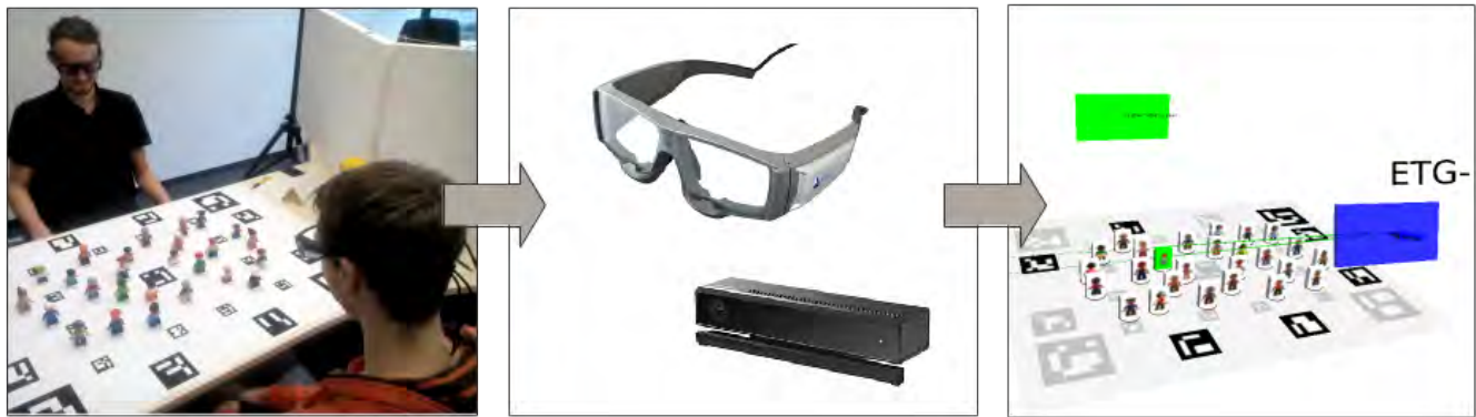
Figure 3: EyeSee3D process: left: real world figure identification task; middle: interaction is tracked using different sensors, such as eye tracker or Microsoft Kinect; right: EyeSee3D fuses tracking data in a 3D situation model including areas of interest for all figures and the heads of the interaction partners (boxes). The picture shows a screenshot from the EyeSee3D preview window for the situation at the left.
