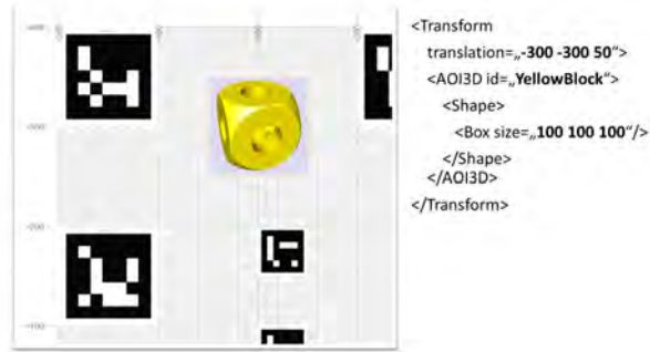
Figure 5: Several coordinate-system templates of different sizes have been designed to help the researcher to link coordinate frames of different devices. The figure shows a larger DIN-A0 paper with a millimeter grid depicting the exact coordinate system that is defined by the augmented reality markers (dark-black patterns) also printed on the paper. A yellow wooden block is used as target stimuli and placed on the template. The coordinates of the AOI can be read from the millimeter coordinate system and transferred to a file describing the 3D situation model for the experiment (right side).
