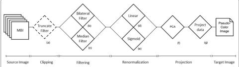
**Fig. 1** Flowchart of the normalization pipeline. Workflow chart of the normalization pipeline for multiplexed bioimages (MBI). The dashed boxes show non-mandatory processes and the solid boxes show mandatory process. For a detailed view, please see the Materials and methods section
