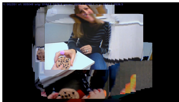
Figure 1: Visualization tool displaying a history of frames with corrected horizontal and vertical camera motion.
