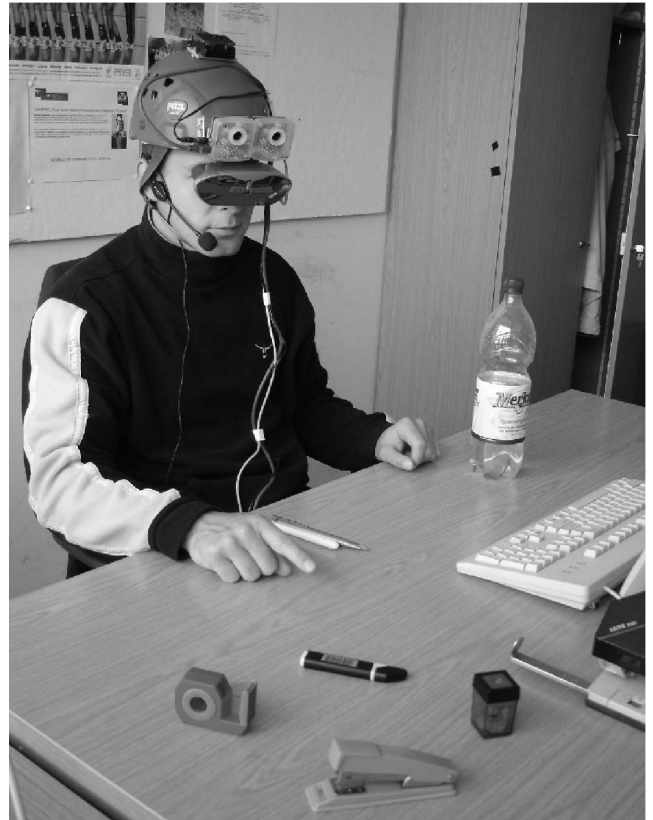
Fig. 1. User with head mounted cameras and display. The input is looped back into the display and enhanced by visual augmentations.
