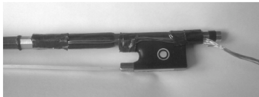
Figure 6.7.: This picture shows the pressure sensors that are attached to the bow. The picture was taken after recording approximately 3000 bowing examples.
