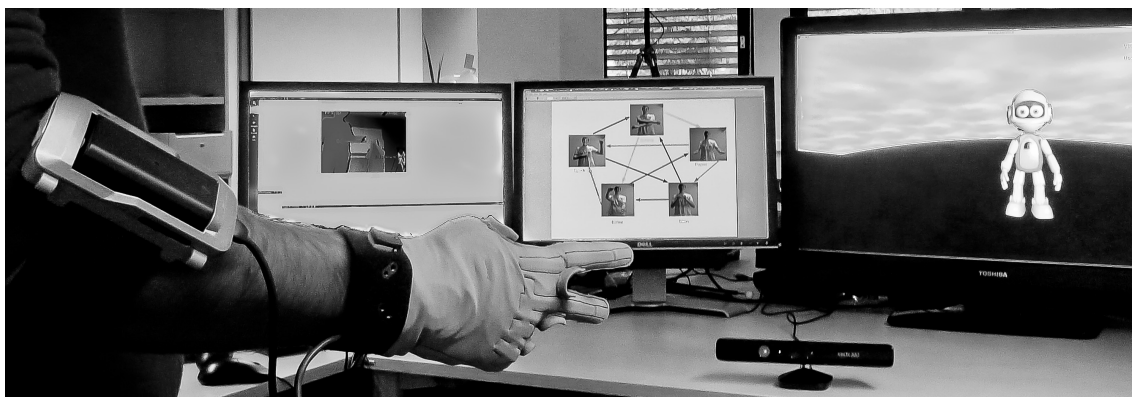
Figure 6.11.: Setup of the RPSLS game; the Microsoft Kinect TM sensor is on a table in front of a monitor on which the virtual agent VINCE is displayed. The leftmost monitor displays the software that captures the Kinect data, the monitor in the middle shows the gestures as a reminder for the player. The arm of the human player wearing a CyberGlove device is in the front.
