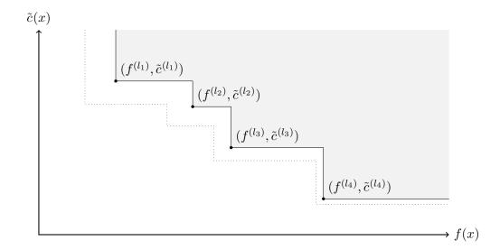
Figure A.2.: An illustration of the filter concept. The filter contains the pairs  $(f^{(l_i)}, \tilde{c}^{(l_i)})$ , i = 1, 2, 3, 4 and the dominated area with respect to Definition 7 is highlighted in grey, i.e. right and above the (including) border determined by the filter pairs. When using the tighter criterion (A.18) the arising border is indicated by the dotted line.
