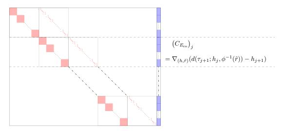
Figure 3.1.: Structure of the Jacobian of the continuity constraints: partial derivatives with respect to h (red) and with respect to  $\tilde{r}$  (blue). White areas contain zero elements.
