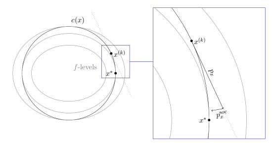
Figure A.3.: Idea of second order correction. In this situation, the current QP approximating the NLP at the (already) feasible point  $x^{(k)}$  determines the direction  $p_x$ . A step of size  $\alpha^{(k,0)} = 1$  along  $p_x$  would lead to a point, which violates the constraints again and even increases the objective. However, a subsequent step along  $p_x^{\text{soc}}$  remedies the problem.
