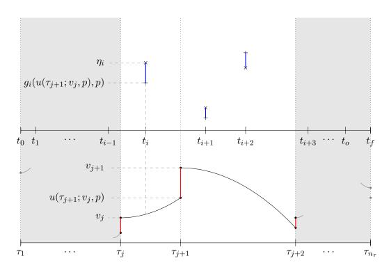
Figure B.1.: Schematic illustration of the multiple shooting approach. The red distance indicates the continuity gap (B.8b), that has to be closed (up to some tolerance); the blue line indicates the residual component of the objective at corresponding measurement times  $t_i \in \{t_1, \ldots, t_o\}$  that has to be minimized.
