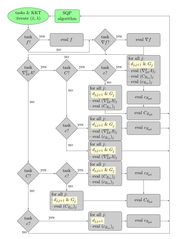
Figure 3.4.: Flowchart of NLP related evaluations (3.8) (grey) depending on a list of SQP tasks and current KKT iterates (green); required IVP solution evaluation  $d_{j,j+1} := d(\tau_{j+1}; h_j, \phi^{-1}(\tilde{r}))$  (3.4) and corresponding sensitivity matrix (3.9) (yellow).
