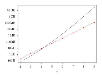
Figure 3.7.: Necessary amount of memory for the dense [17] (black crosses) and our sparse (red bullets) datastructure to persist  $\Theta$ .
