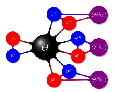
Figure 3.6.: Illustration of the concept of implementation for  $\Theta$ . Structural elements are indicated in blue, data elements in red and coefficient matrices in purple. When  $\Theta$  has to be updated, first,  $\langle r \rangle$  is calculated with respect to W, followed by  $\theta^{[k]}$  with respect to  $\Theta^{[k]}$ . Afterwards,  $\Theta^{[k]}(r)$  can be used in the linear map provided by (3.11).
