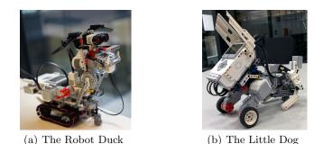
**Fig. 2.** Two examples of the different robots created by the project groups. Image (a) shows robot duck with ears to show emotions. Image (b) shows a dog like pet with eyes presented on the display.
