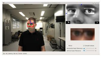
Fig. 2: Gaze tool displaying detected eye regions (top right), pupil positions, gazing angles (blue) and mutual gaze detection (red).
