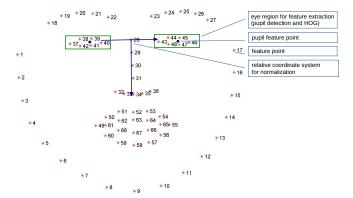
Fig. 3: 68 point feature points markup [17] with annotated features and regions used by our system.
