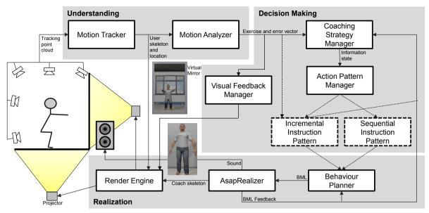
Figure 3: The overall architecture of our intelligent coaching space. On the left the hardware setup is depicted, with wall and floor projection and motion capturing cameras. In our software we have understanding components interpreting the user's actions. Our decision makers comprise both visual feedback (middle part) and a virtual coach and realization components to communicate the decisions back to the user.
