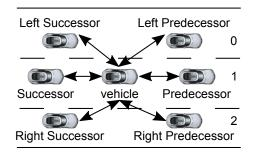
Figure 4.4: Car-to-car relations. Relations between a vehicle and its surroundings.
