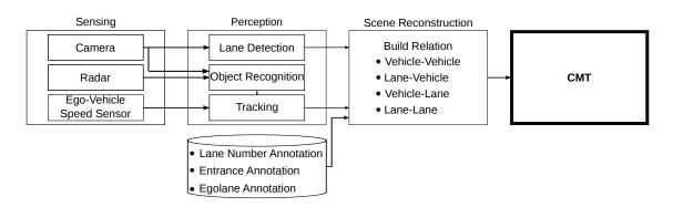
Figure 4.3: Overview of the system architecture for lane change behavior prediction.
