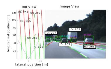
Figure 4.16: Example of a scene for which the model "Entrance Giveway" is wrongly active. The left part shows the BEV, the lane markings and the radar targets with their relative velocity. The scene on the right shows that vehicle 268, being driving in the giveway lane, will change lane to overtake the truck in front of it, not because of a vehicle on the entrance lane.
