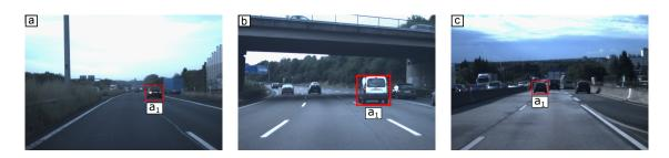
Figure 4.9: Three exemplary scenes where vehicles being driven in the left neighboring lane of the entrance on the highway and change lane to the left because of entering vehicles.
