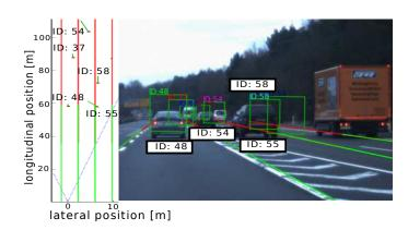
Figure 4.14: Example of a scene for which the model "Entrance Enter" is wrongly active. The left part of this image shows a bird's-eye view (BEV) with the ego-vehicle at the x-position 0, the lane markings and the radar targets with their relative velocity. The scene on the right shows the current scene in which vehicles 55 and 58 are assigned to the wrong lane because of the zebra area.
