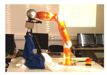
Fig. 1: Case study: automated gripping of laundry with the KUKA Lightweight Robot IV.
