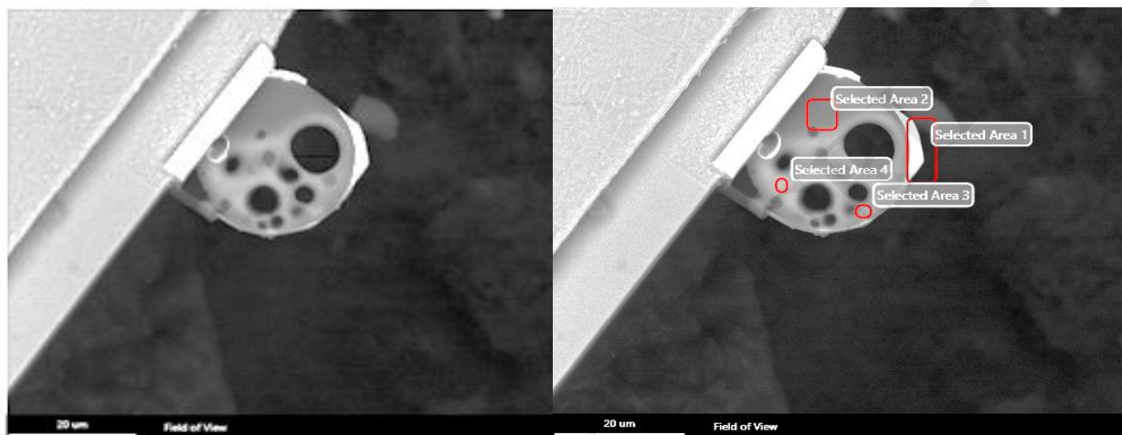
Figure 9: Left BSE image showing the various regions and voids in the PMC Zapper particle, and right, the regions examined via EDS analysis.
