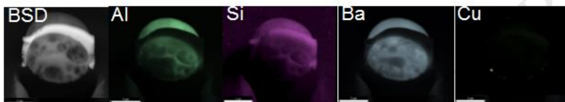
Figure 7 - EDS maps of FIB sectioned particle from 0.40 Winchester Winclean ammunition. (L to R - Backscattered electron image, Al map, Si map, Ba map, Cu map)
