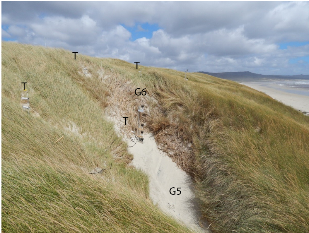
Figure 11: G6 mast location at the base of the cauldron's vertical scarp, with G5 location indicated in the foreground and Hilton traps also indicated (T). Note the highly complex 3-D flow structure within the slot and cauldron as indicated by the bending directions of the Ammophila vegetation.
