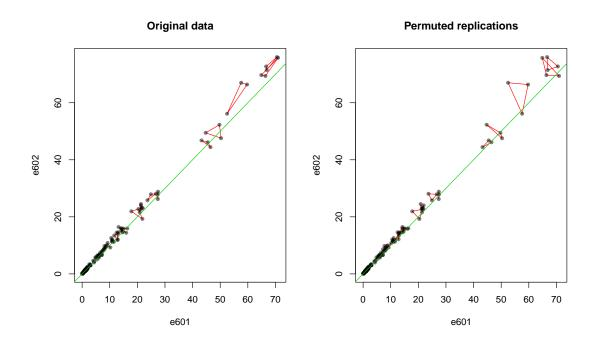
Figure 5.10: Example 2. Scatter plot for measurements of system e601 vs. system e602. Left: original data, right: data with randomly permuted replications. The replications are connected with red lines.
