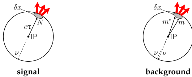
Figure 37: Shown is a schematic illustration of the signal signature and a possible SM background. The signal arises from the decay of a long-lived heavy neutrino with mean lifetime \tau . While for the SM background, the merger of two secondary vertices is considered which arises from long-lived mesons m and m^* that decay sufficiently close to each other such that only one secondary vertex can be resolved. The detector resolution \delta x depends on the detector component. This figure has been published in ref. [2].
