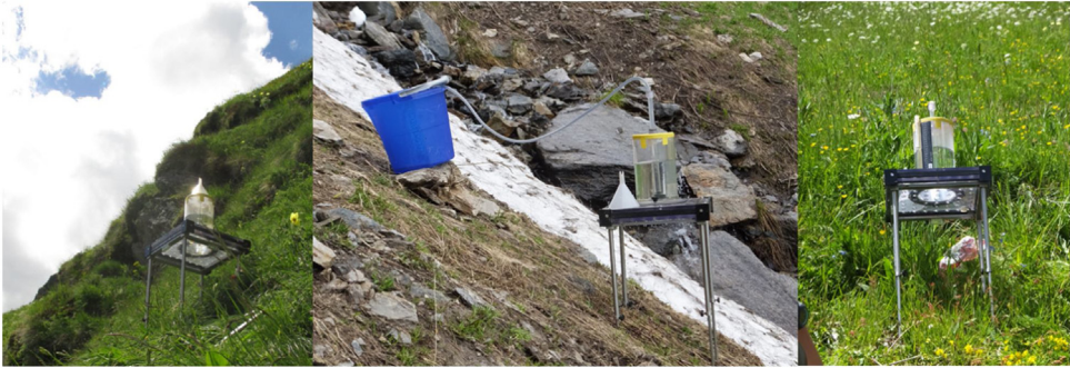
Fig. 1. Different set ups and preconditions of the rainfall simulation experiment on steep slopes in Val Piora, Ticino, Switzerland.
