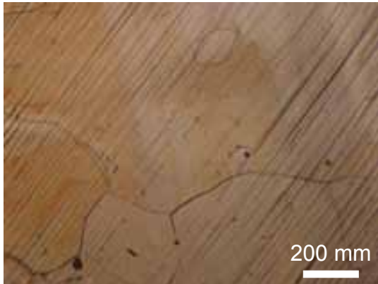
Figure 5.4. (a) Optical microscopy image of a CVD grown monolayer hBN film on a Cu foil before and after a heat treatment. The color contrast is enhanced for a better visibility.
