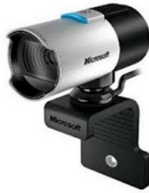
Figure 2. The picture of the webcam with CMOS sensor used as a detector.
