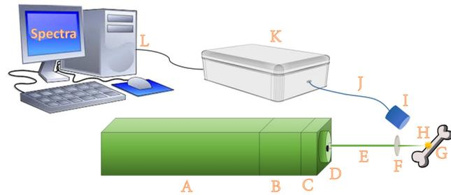
**Fig. 1** Schematics of the LIBS setup: A, laser (flash-lamp-pumped Nd:YAG), B, second-harmonic generator; C, harmonic separator; D, beam blocker; E, laser beam; F, focusing lens; G, bone sample; H, generated plasma; I, light collector; J, fiber optic; K, spectrometer (echelle); and L, computer.
