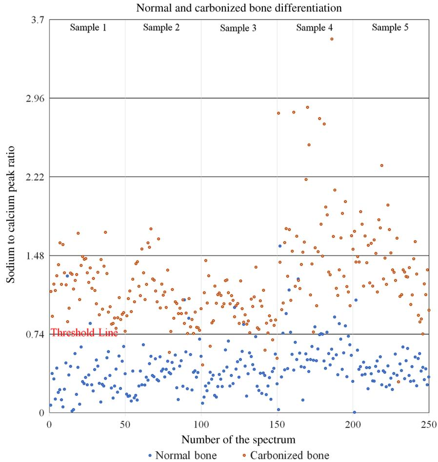
Fig. 4 Sodium-to-calcium intensity ratio for all samples.
