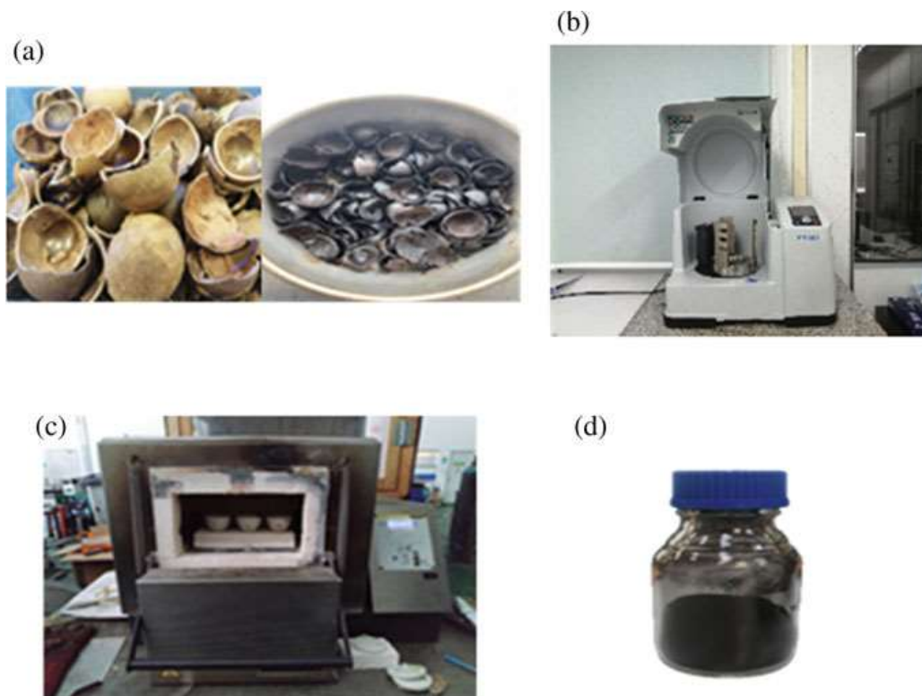
Fig. 2 Synthesis process for nano-activated carbon (NAC); a Dried and charred Tamanu shells, b ball-mill machine, c activation process and d nano-activated carbon powder
