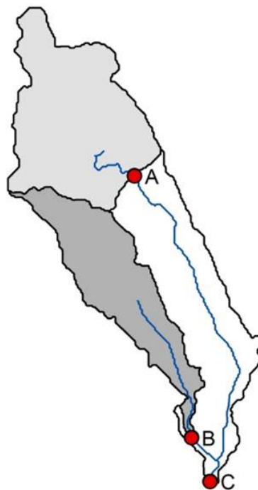
Figure 3. Example of the export calculations for connected catchments. The DOC contribution from the downstream catchment represented by the white area was calculated by subtracting the exports from upstream catchments A and B from the export calculated at the downstream catchment C.
