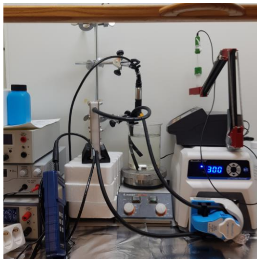
Figure A3. Shows the set up used in to treat PFASs in Millipore, DOC and Membrane reject water.
