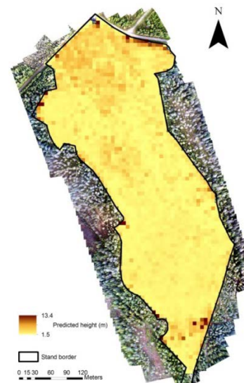
Figure 9. Predicted tree height, using the metric Elev_P20, for a stand (number 1 in Table 2) that is not in need of cleaning. Darker color indicates higher objects.
