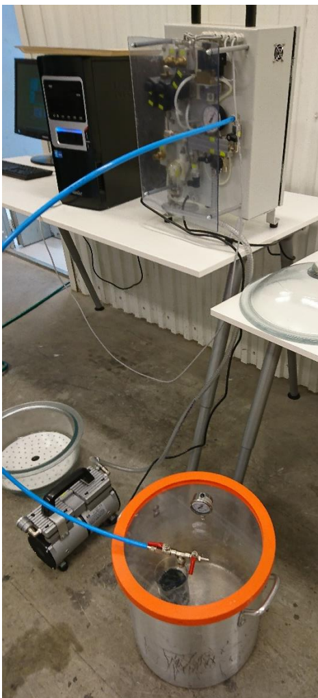
Figure 5: The VI setup at OptiFreeze. To the far left is the computer which is connected to the vacuum pump and on the floor, is the chamber. Photograph: Maria Hellström.
