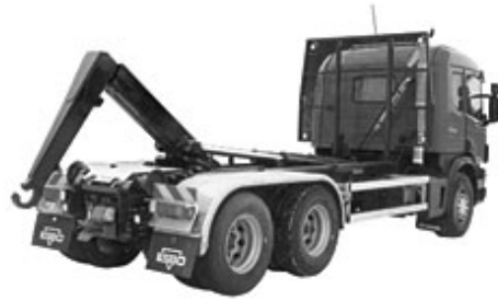
Figure 15 Self-discharging lorry fitted for handling swap bodies
