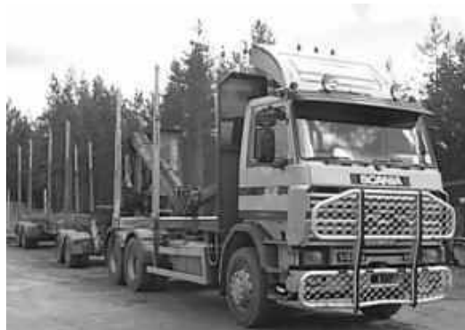
Figure 16 Timber lorry with on board crane
