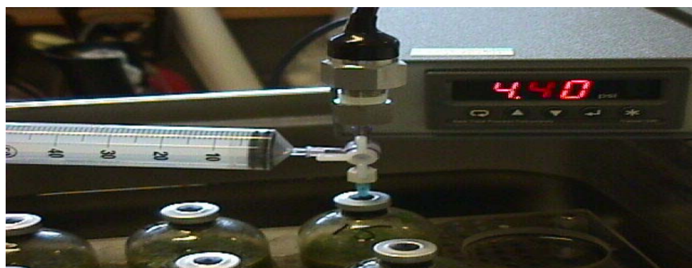
Figure 4. The pressure transducer connected to a digital display measuring gas pressure and volume of fermentation gas.
