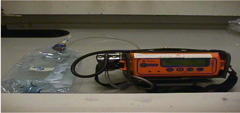
Figure 5. A H 2 S meter connected to a plastic bottle filled with fermentation gas and 800 ml CO 2 .
